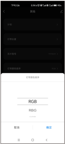
灯带颜色顺序界面 根据灯带的颜色顺序选择对应的R/G/B/W顺序。(RGB, RBG, GRB, GBR, BRG, BGR, RGBW, RBGW, GRBW, GBRW, BRGW, BGRW, WRGB, WRBG, WGRB, WGBR, WBRG, WGBR)
